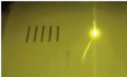
Melting of metallic powder by CO2 laser
